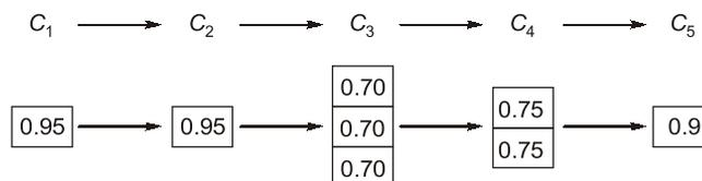
Because of the low reliability of the third and fourth components, they are replicated, the system now contains 3 of the third component and 2 of the fourth component. What is overall system reliability?
