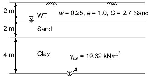
Unit weight of the partially saturated sand above the water table.
