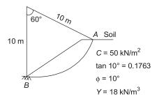
Normal effective pressure on sliding surface AB is 255 kN/m<sup>2</sup> downward tangential disturbing force along AB is 840 kN.
