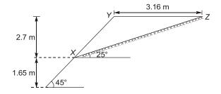
The FOS against wedge failure along the interface is
