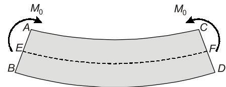
**NOTE :** In plastic bending neutral axis passes through equal area axis. Equal area axis may be different from centroidal axis or may coincide with centroidal axis which depends upon shape of cross-section.
