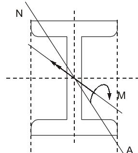
**NOTE:** Under unsymmetrical bending, plane of bending and plane of couple are not same whereas in case of symmetrical bending plane of couple and plane of bending are same.
